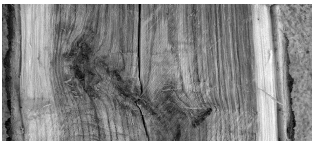
Figure 3. Sound knot after artificial pruning, fully occluded with small bark pocket. Sound wood tissue around knot.
