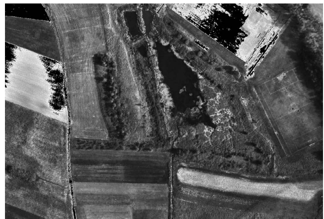
Figure. 640 nm optical band, altitude 1200 m, FLAASH algorithm processed image, scale on image 2
