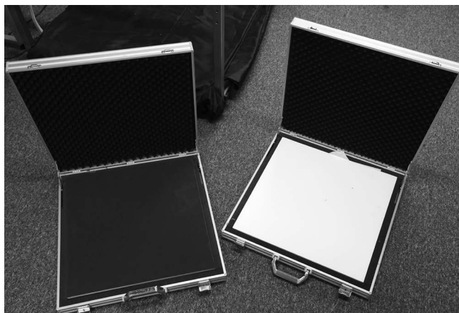
Figure 2. Low (<5%) and high (>95%) reflectance in visual and near infrared light calibration markers used in HESOFF project
