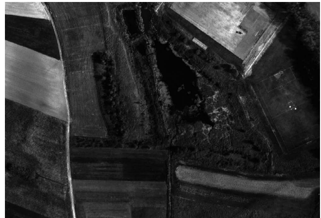
Figure 5. 640 nm optical band, altitude 1200 m, QUAC algorithm processed image, scale on image 2
