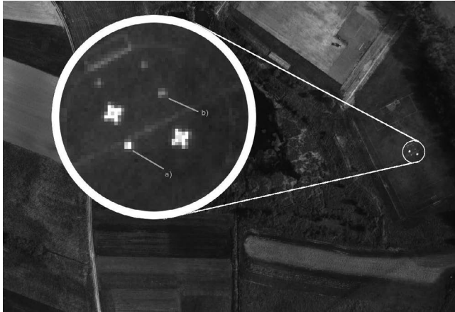
Figure 1. Calibration markers with (a) >95% and (b) <5% reflectance photographed from altitude 800 m
